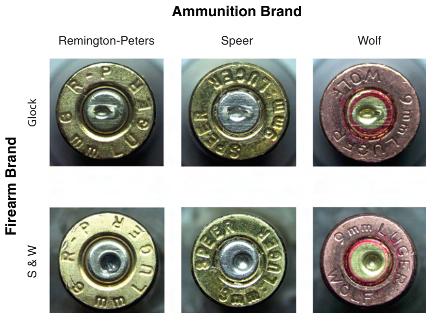
FIGURE 2-2 Breech face markings and firing pin impressions for three ammunition types and two firearm brands.
