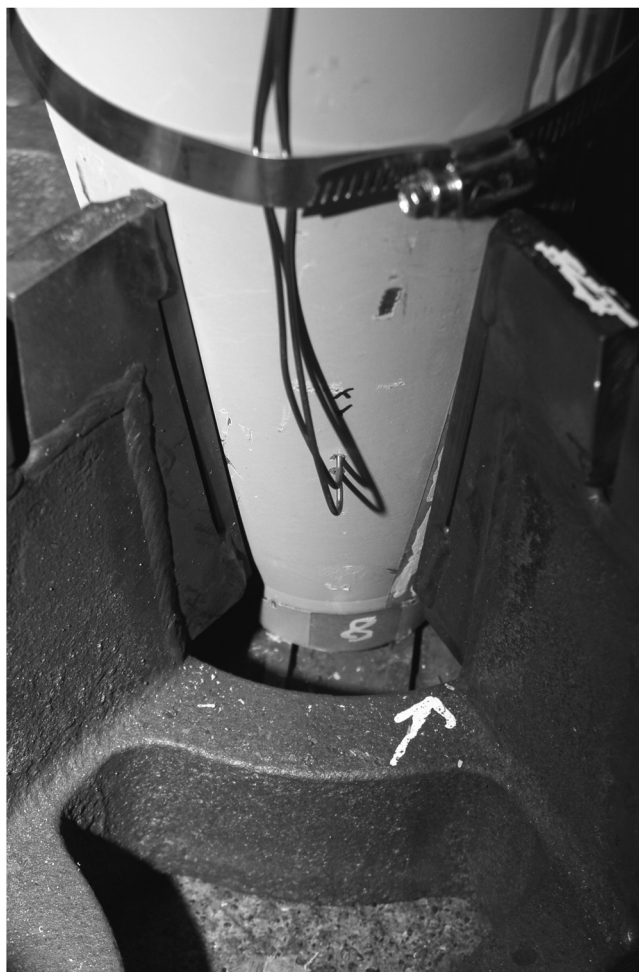
FIGURE 4-3 Thermocouple installation on the projectile. SOURCE: BPBGT, 2007a.
