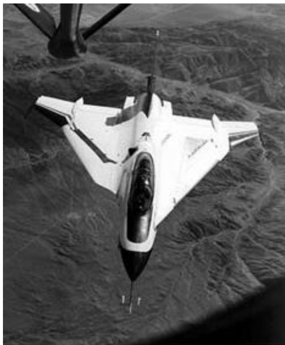
FIGURE 3.2 NASA laminar flow flight test vehicle at the Dryden Flight Research Center. SOURCE: NASA Langley Research Center Web site at http://128.155.35.117/LFC_www/LFC.html .
