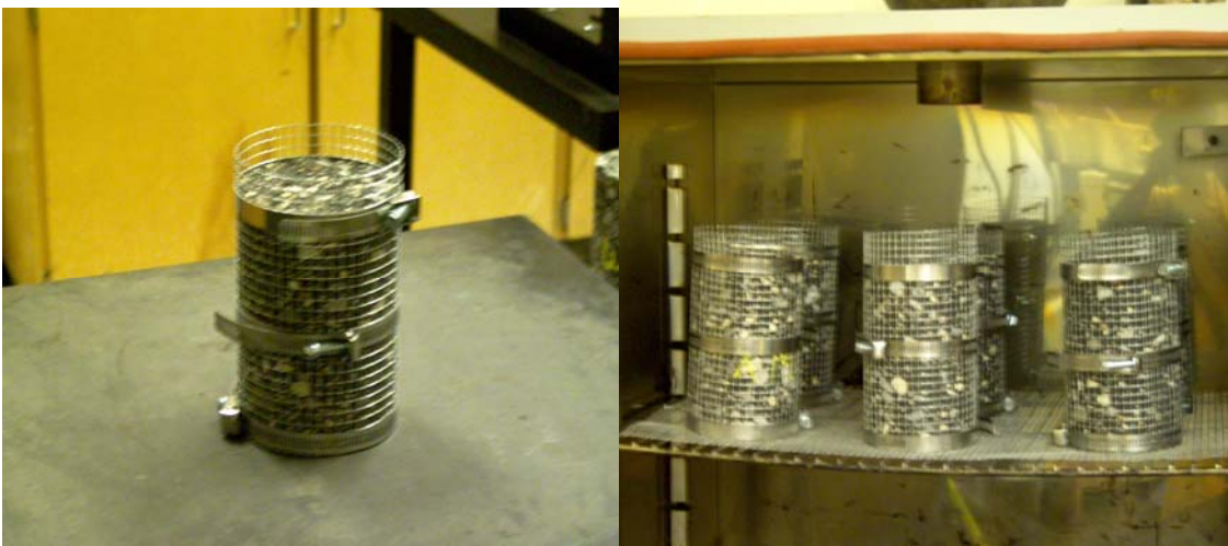
Figure 125 E* Test Cores Encased in Wire Mesh and Clamps to Eliminate Slump During Aging
