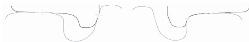
(c) Flangeway width 1.613 in. (optimal).
