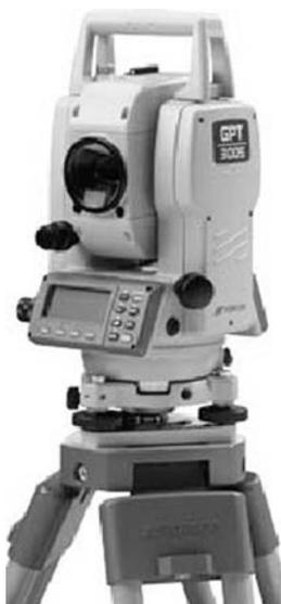
FIGURE 17 Total station survey device.
