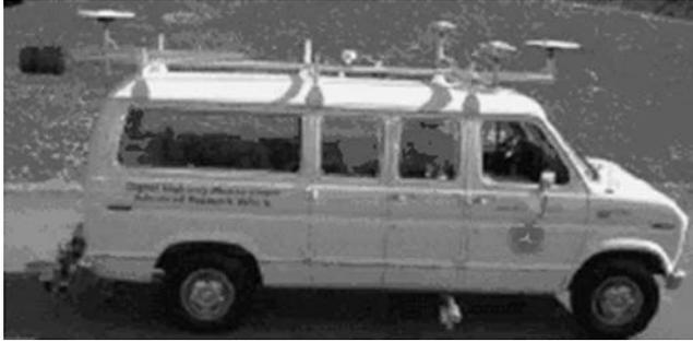
FIGURE 19 FHWA–Turner–Fairbank Highway Research Center digital highway measurement vehicle.
