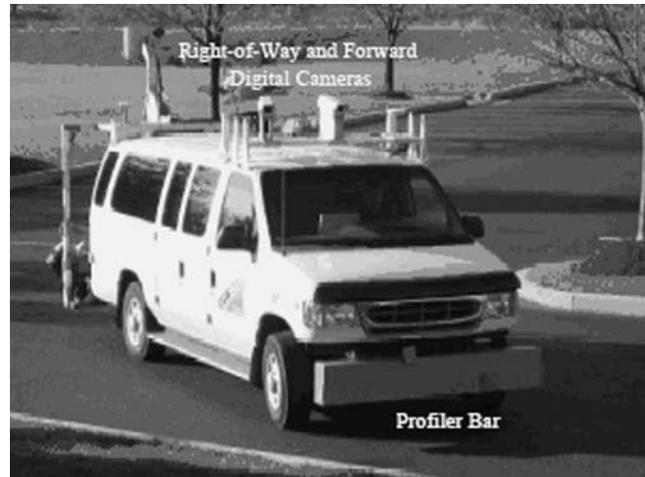
FIGURE 18 Road inventory vehicle with digital cameras and road profiling system (46).
