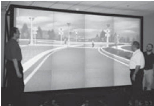
Visual analytics display for collaboration and sharing of visual information by transportation researchers and users. Imagery is from a 3-D model of alternative roundabout treatments under consideration by National Cooperative Highway Research Program (NCHRP) Project 3-78, Crossing Solutions for Visually Impaired Pedestrians at Roundabouts and Channelized Turn Lanes. The imagery was developed in collaboration with Thomas Fischer, New York State Department of Transportation (DOT). Several static views from driver and pedestrian vantages are available for online review at www.itre.ncsu.edu/NCHRP378/ .
