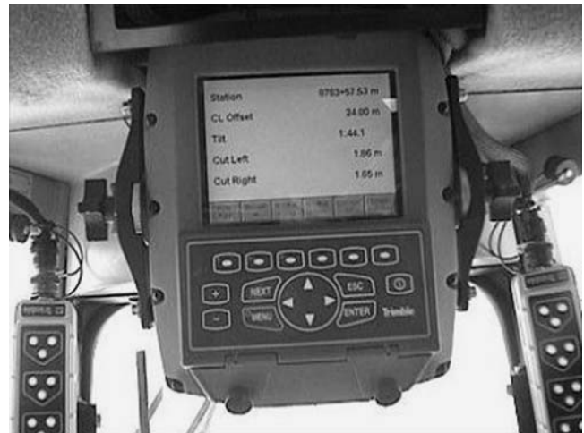
FIGURE 20 Cab-mounted GPS computer with light bars (Courtesy: McAninch Corporation).
