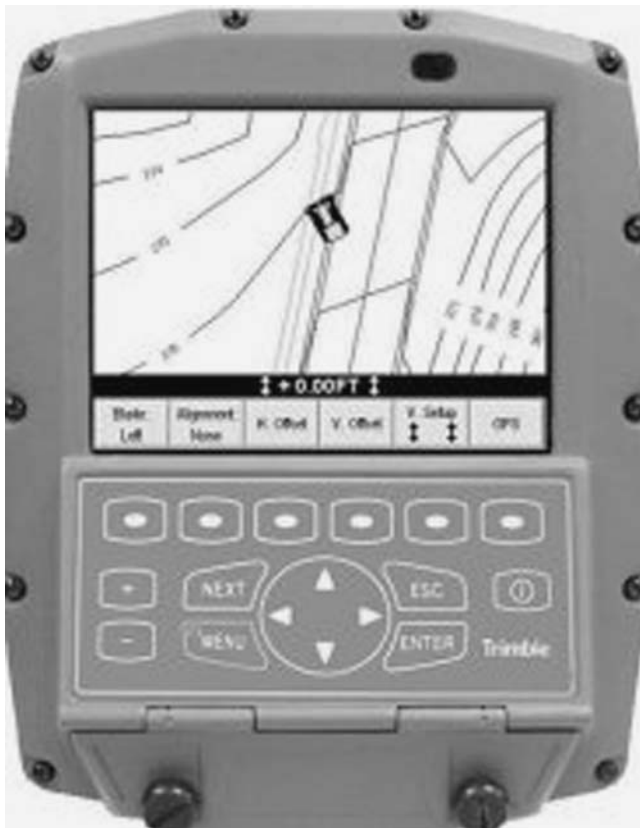
FIGURE 19 Machine-mounted GPS computer (Courtesy: McAninch Corporation).
