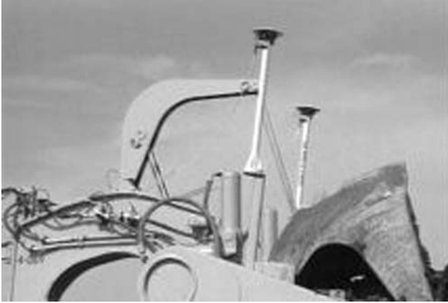
FIGURE 12 Dual GPS antennae on scraper pan (Courtesy: McAninch Corporation).
