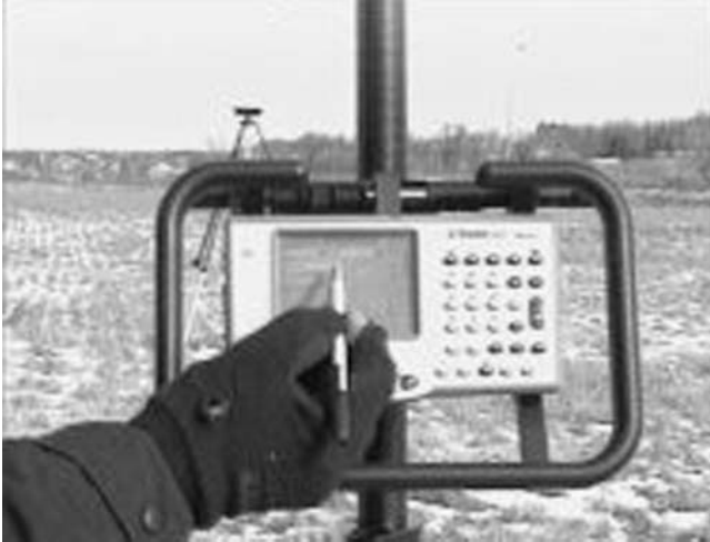
FIGURE 8 GPS field computer and stylus input (Courtesy: McAninch Corporation).
