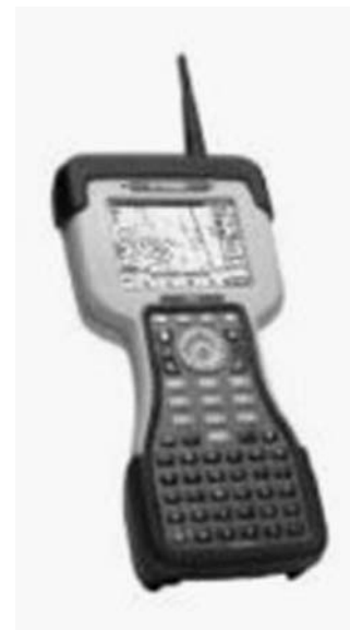
FIGURE 22 GPS rugged handheld computer (Courtesy: McAninch Corporation).
