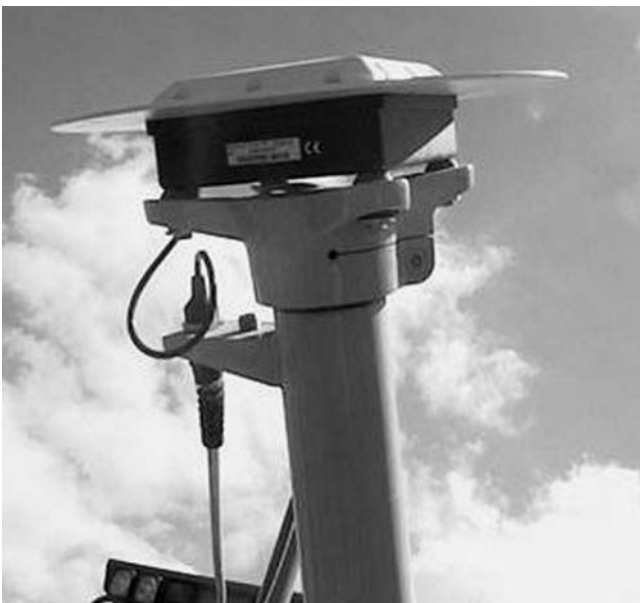
FIGURE 14 GPS antennae close-up (Courtesy: McAninch Corporation).
