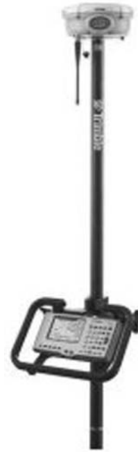
FIGURE 6 GPS antennae and computer (Courtesy: McAninch Corporation).
