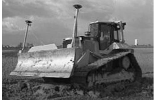
FIGURE 15 Dual GPS blade antennae on dozer (Courtesy: McAninch Corporation).
