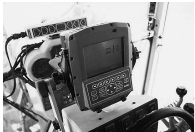
FIGURE 21 Machine-mounted GPS computer (Courtesy: McAninch Corporation).
