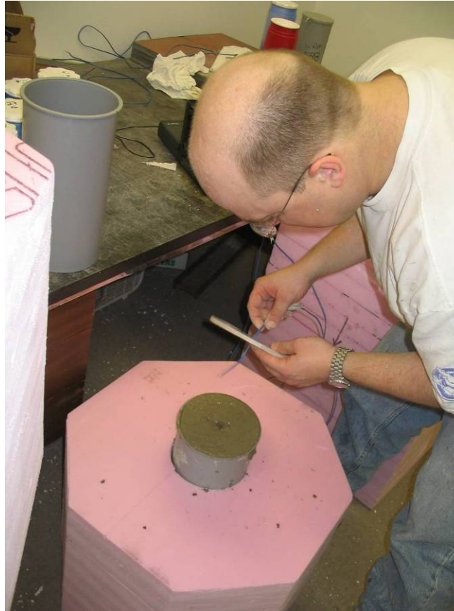
Figure A-7. A thermocouple was placed in the center of each concrete cylinder
