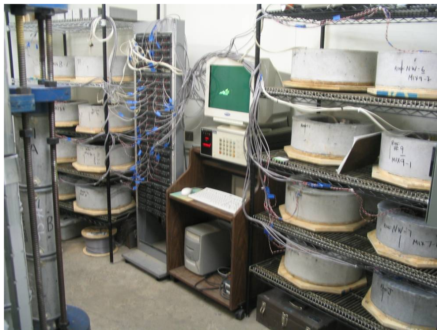
Figure A-5. Ring storage and data collection in 50% RH laboratory environment
