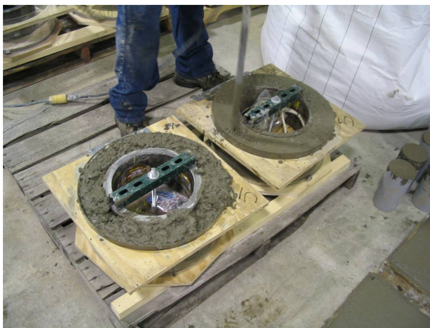
Figure A-4. Rings being cast and vibrated for cracking tendency test
