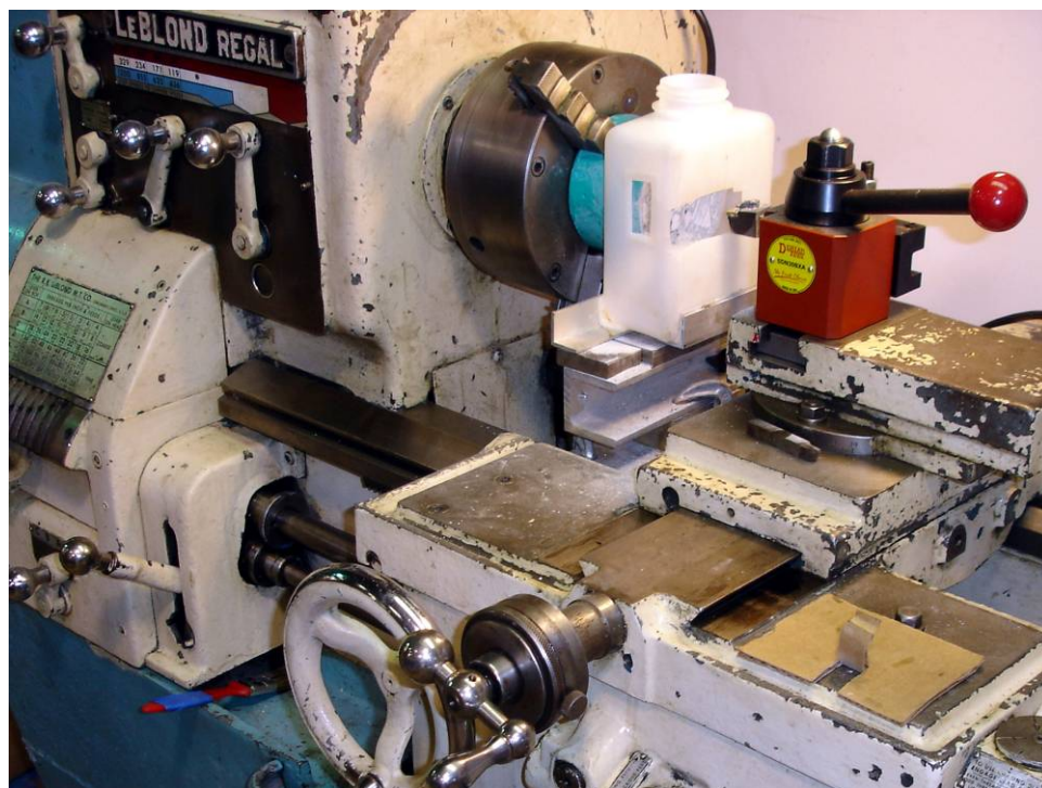
Figure A-21. Lathe used to mill surface of concrete cylinder
