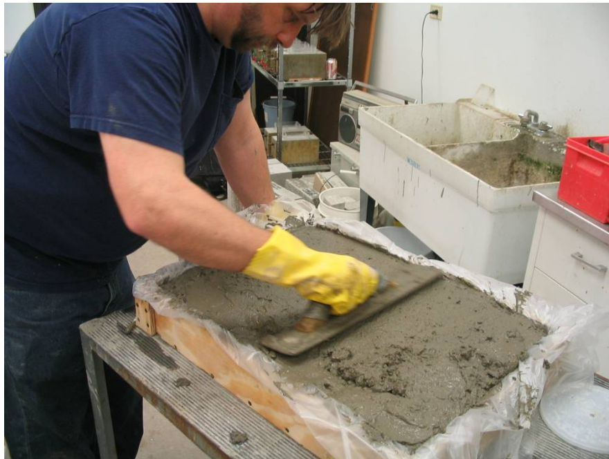
Figure A-2. Performing finishability test on concrete mixture
