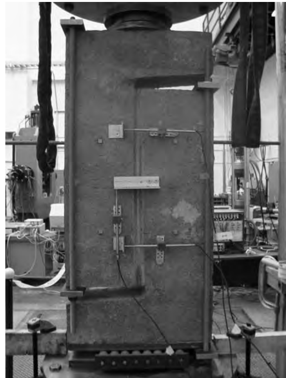
Figure 105. Shear friction test set-up.
