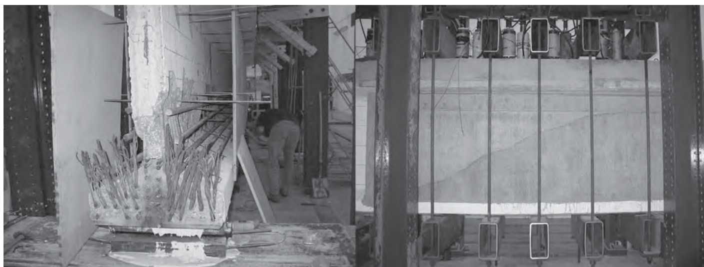
(a) Failed end region before repair
