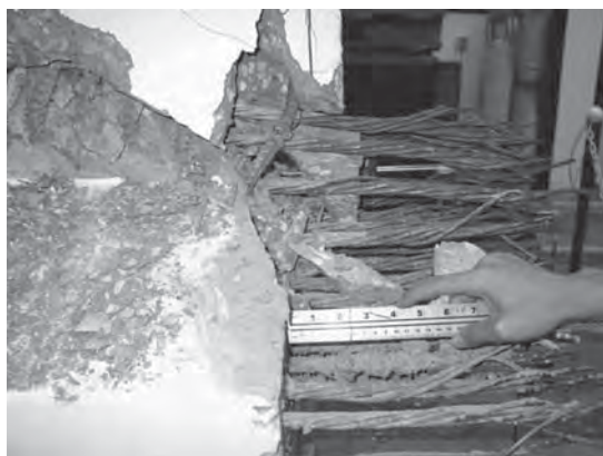
(e) Horizontal shear slip
