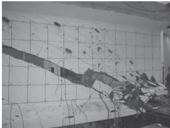
(a) Low v/f'_c , stirrups yield and rupture
