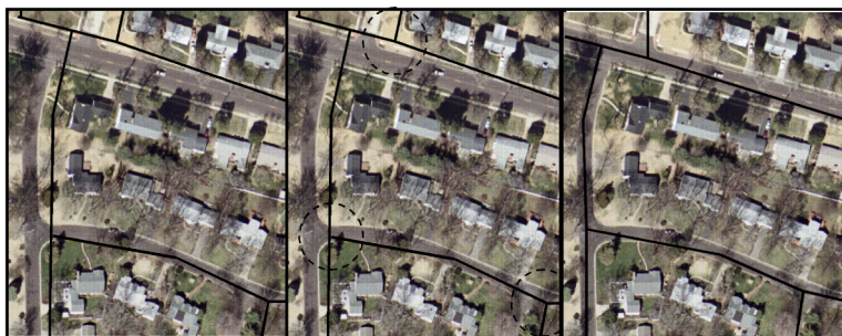
FIGURE 3.10 Automatic conflation of road vector data with imagery. This illustration depicts the conflation process applied to an orthophoto and street centerline file. After the identification of key registration points (street intersections) by the circles, the street line file is spatially aligned with the orthophoto. The right-hand illustration shows the corrected images. SOURCE: Knoblock and Shahabi (2007); used with permission.
