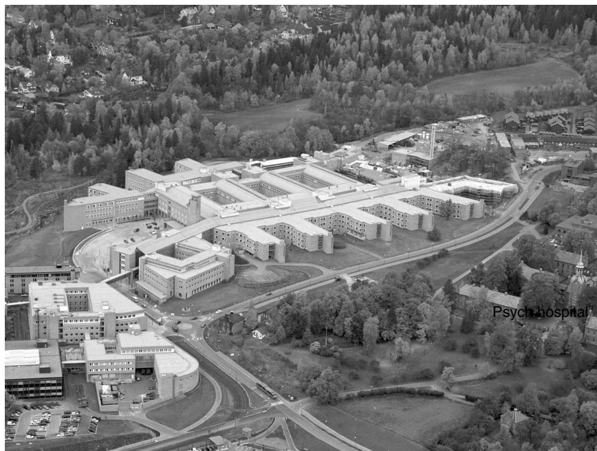
FIGURE 2-3 This hospital’s architects focused on designing a humanizing environment, not minimizing the footprint. The main street is the backbone of the hospital and encourages informal meeting between staff. Walkways connect patient units with treatment facilities.
