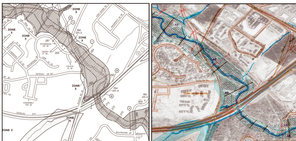
FIGURE 3.5 Comparison between paper and digital FEMA map panels (FEMA, 2006c). The left panel shows an older, paper map; the right panel shows a digital version of the same area.
