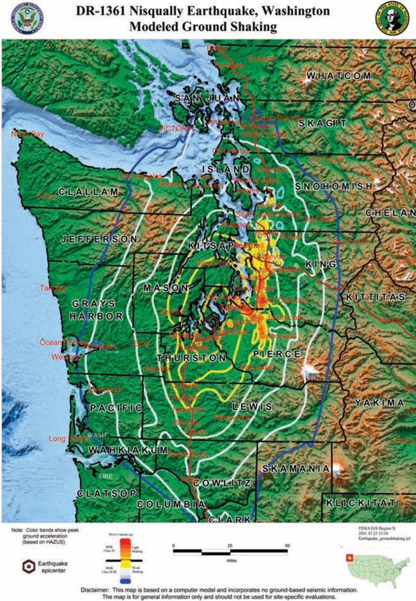
FIGURE 4.1 Example of modeling of ground shaking in the northwestern United States. Courtesy of the Washington State Emergency Management Division and the Federal Emergency Management Agency.
