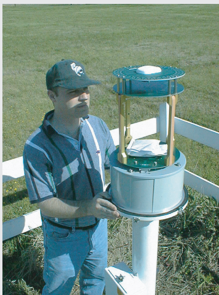
A lightning sensor with the top removed showing the crossed loops that detect the azimuth to a distant lightning flash.
