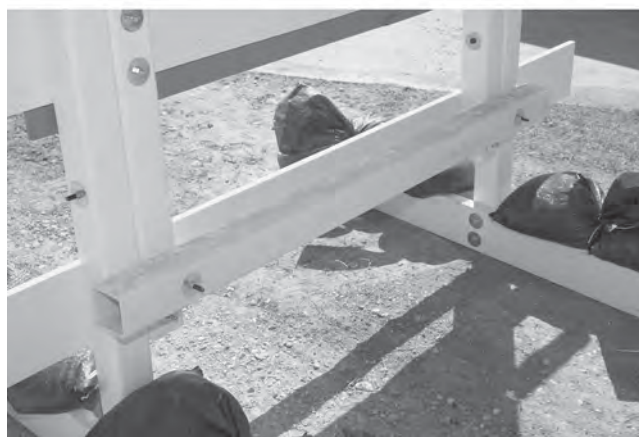
Figure 6.23. Hollow-HDPE/wooden barricade with rectangular sign used for Test 4.
