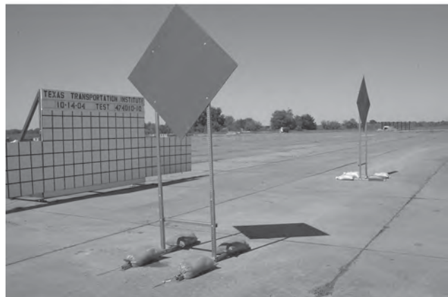
Figure 8.23. Dual uprights with raised slip joint before Test 10.
