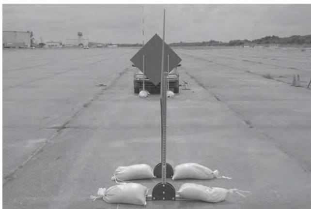
Figure 7.15. Pivoting dual-upright system used in Test 6.
