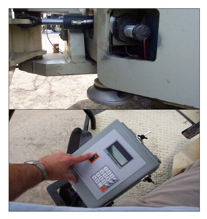
FIGURE 6 Roller-mounted PQI density measuring device and operator display unit
