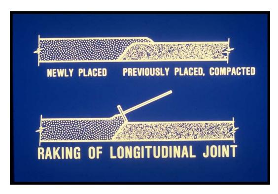
FIGURE 4 Placement of material on hot side of joint.
