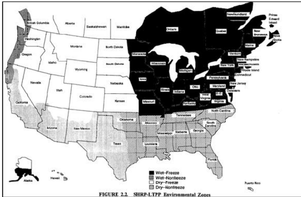
Figure 4: Climatic regions as defined by the Longterm Pavement Program.
