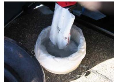
Figure 13. Ice Poured Into PVC and Plastic Bag.
