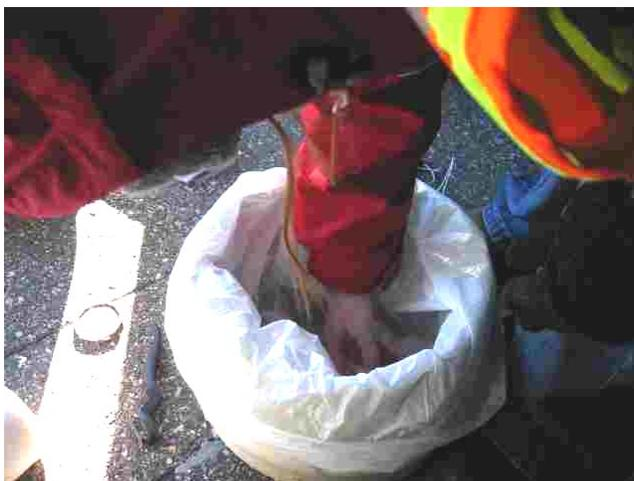
**Figure 22. Field Method for Establishing Ice Bath - Place Plastic Bag Over PVC Section**
