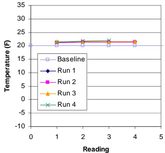
**Figure 37. Passive Sensor Results with Sensor A Using a 10 Percent Sodium Chloride Solution**
