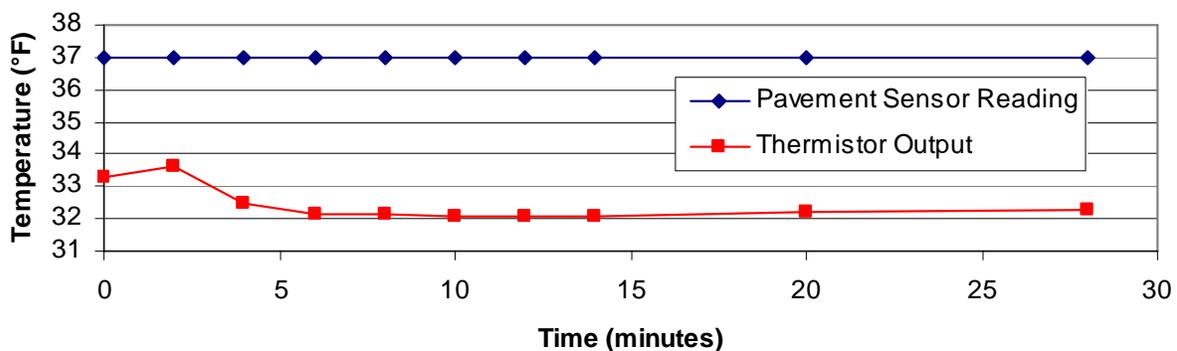
**Figure 27. Sensor C Ice Bath Field Test**
