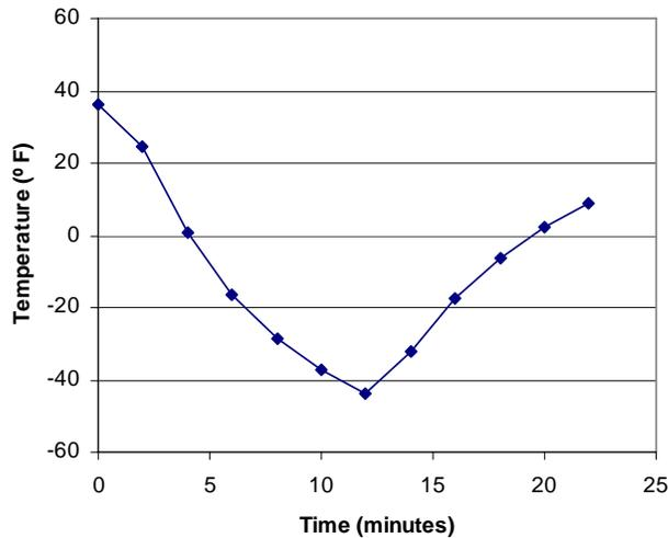
**Figure 34. Graph Showing Temperature Recovery of a Sensor after the Dry Ice Test**
