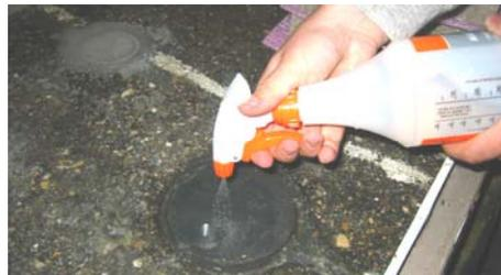
**Figure 10.** *Spraying Tap Water on the Sensor Surface.*
