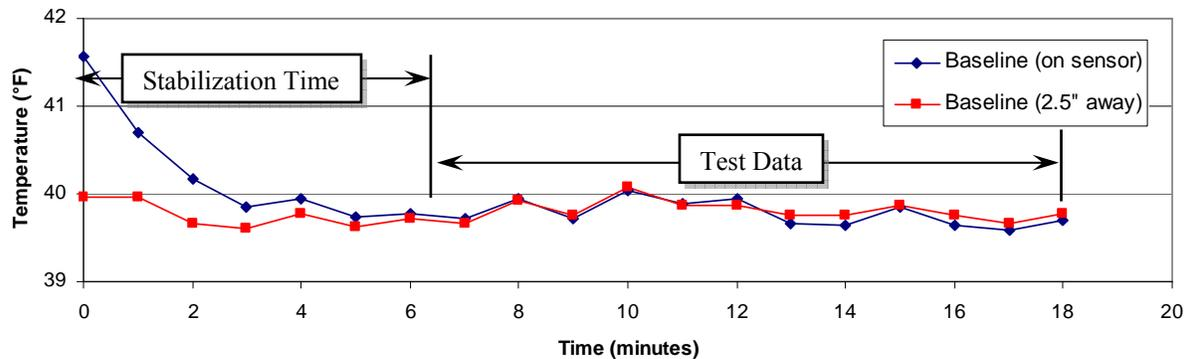
**Figure 18. Graph Showing Effect of Water Film Cooling on the Pavement Section in Laboratory Test**
