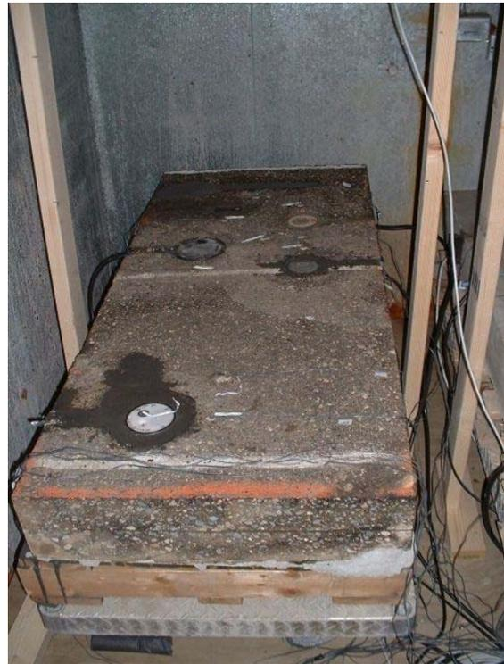
**Figure 11. Asphalt Test Section Installed in Environmental Chamber**
