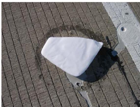
*Figure 6-2. Dry Ice Resting on Pavement Sensor.*
