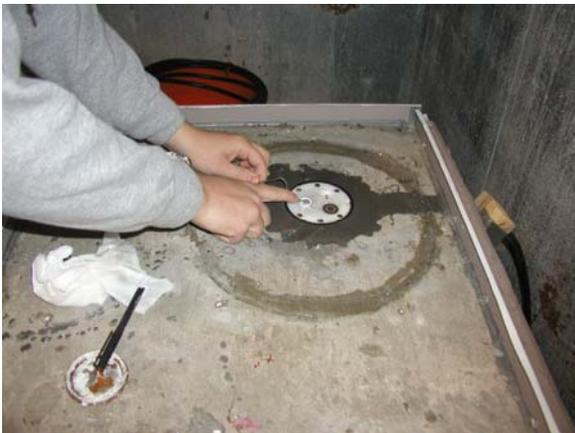
Figure 2-1. Applying Thermal Paste to Sensor
