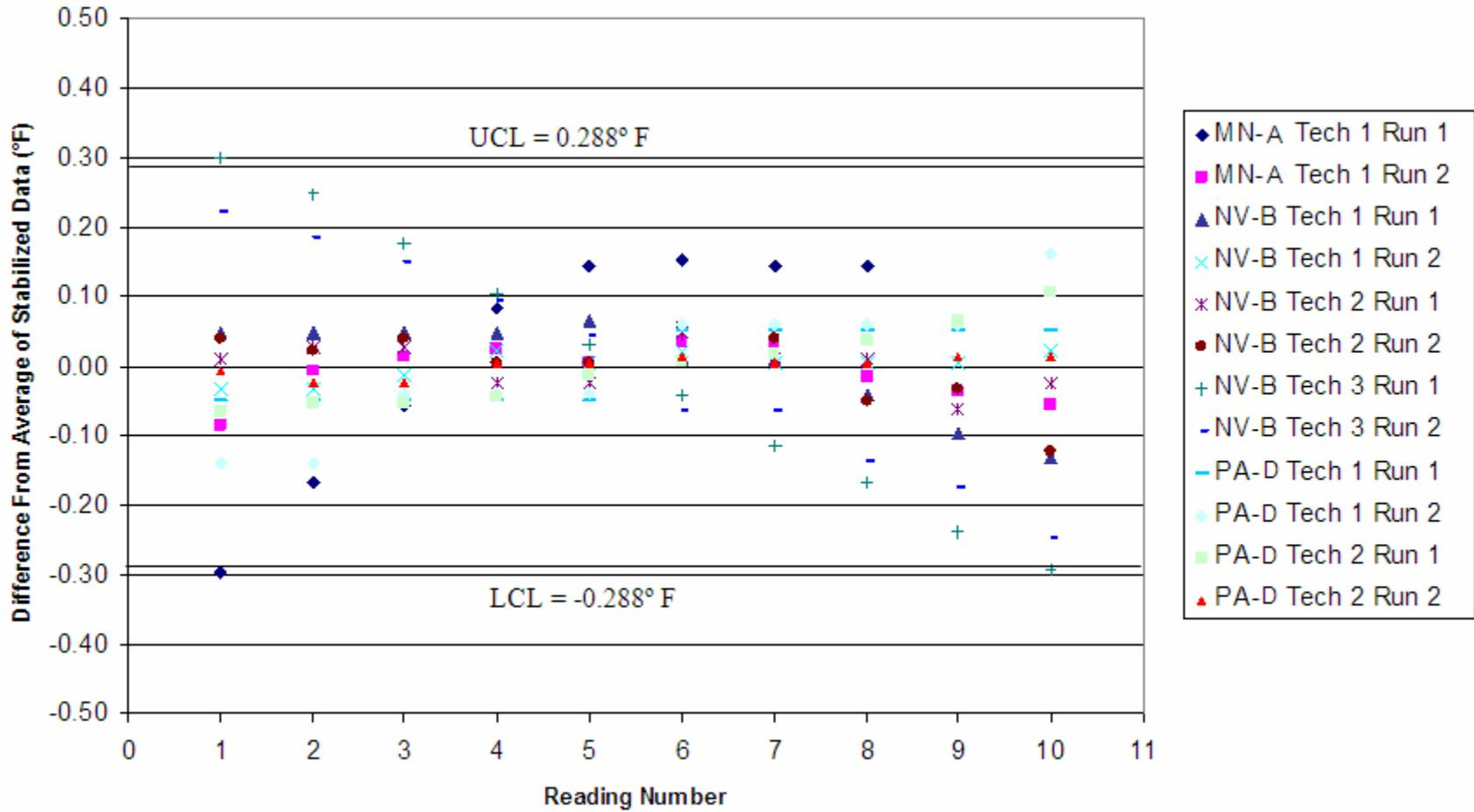
Figure 4. Run Chart for Statistical Process Control of Pavement Temperature for Field Tests
