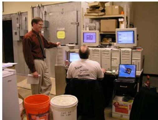
**Figure 13. Data Acquisition System Outside Environmental Chamber Used in Laboratory Tests**
