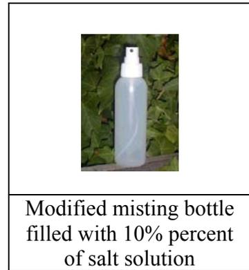
Modified misting bottle filled with 10% percent of salt solution
