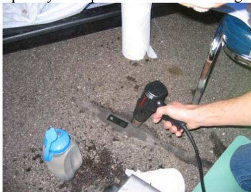
**Figure 35. Drying a Pavement Sensor with a Heat Gun**
