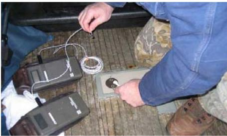
**Figure 7. Applying Thermal Paste to Sensor.**
