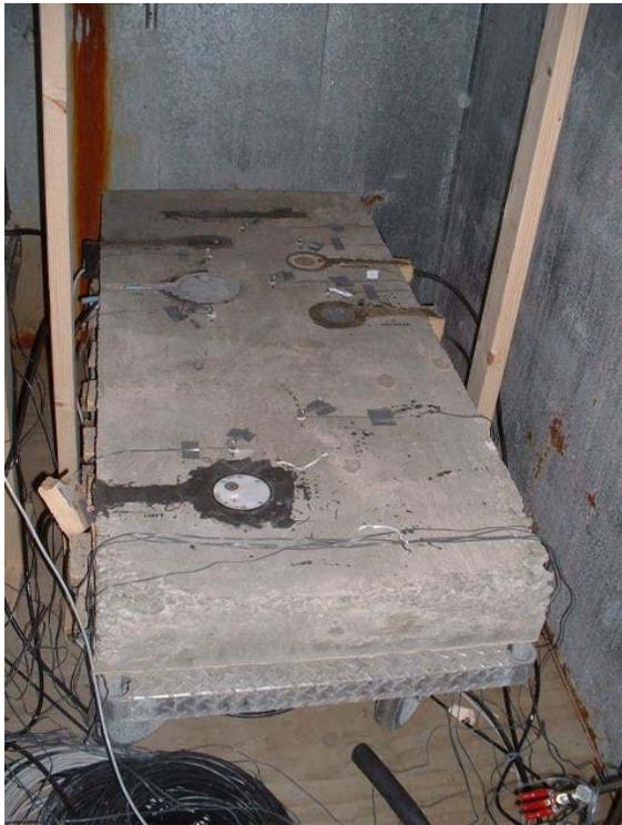
**Figure 10. Concrete Test Section Installed in Environmental Chamber**
