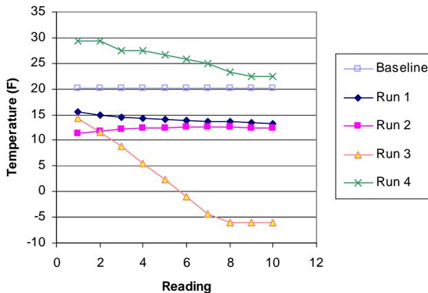
**Figure 42. Passive Sensor Results with Sensor B using a 15 Percent Sodium Chloride Solution**
