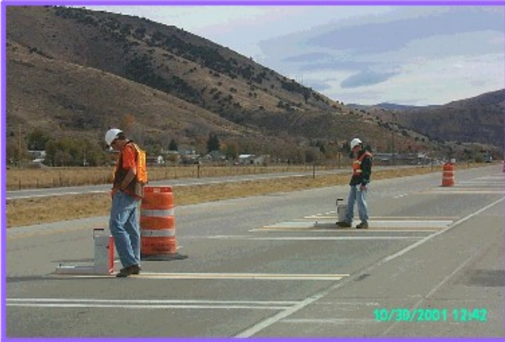
Figure 6. Retroreflectivity measurements on the left wheel path and centerline(25)
