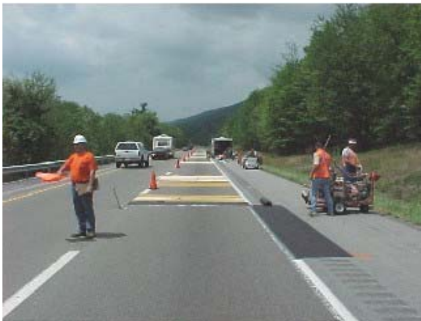
Figure 4. Typical set-up for field tests using test decks. (24)
