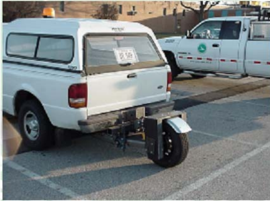
FIGURE 4 Tow hitch unit.
