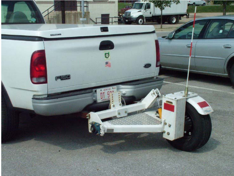
FIGURE 10 Offset tow unit.
