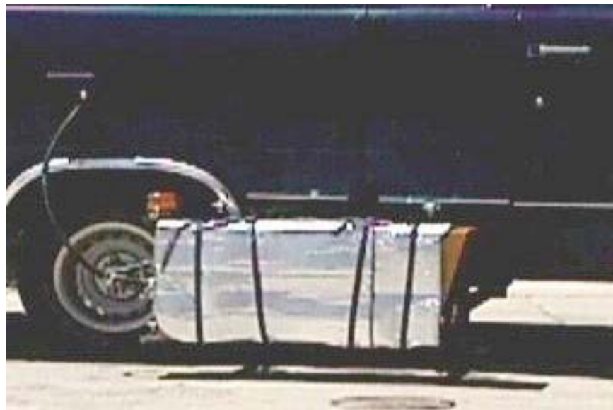
FIGURE 1 Laserlux mobile retroreflectometer mounted on a van.
