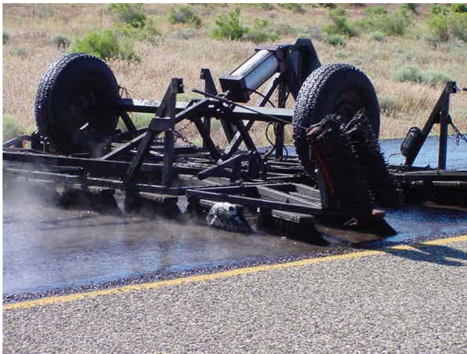
FIGURE 8 Redesigned hydraulic control scrub broom eliminates excess emulsion at seal edge.
