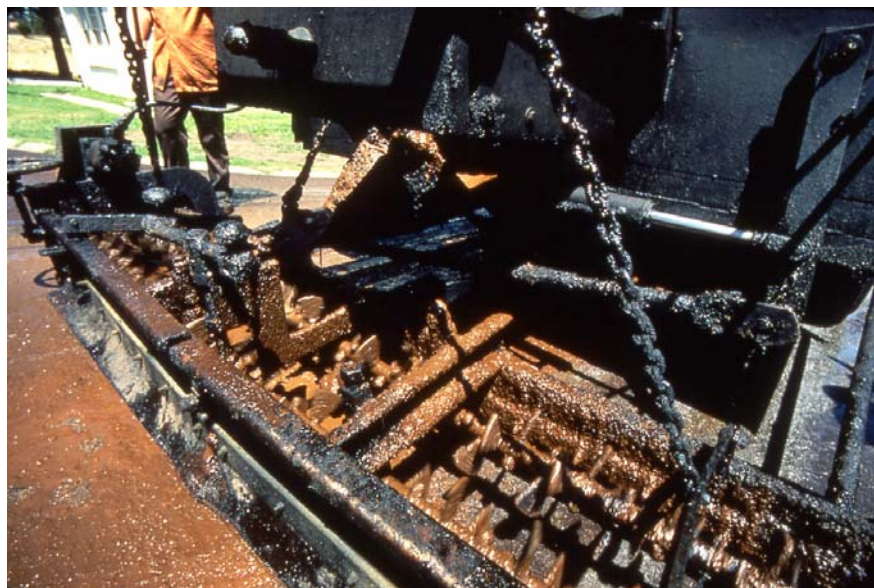
FIGURE 13 Augered laydown box on microsurfacing machine.
