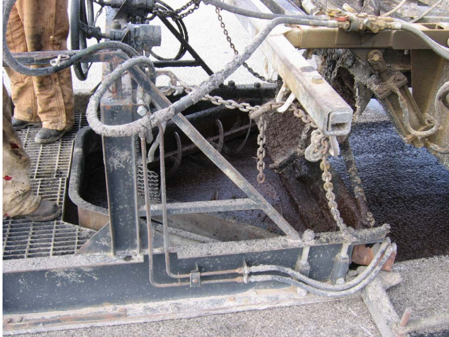
FIGURE 15 Rut-filling box on microsurfacing machine.
