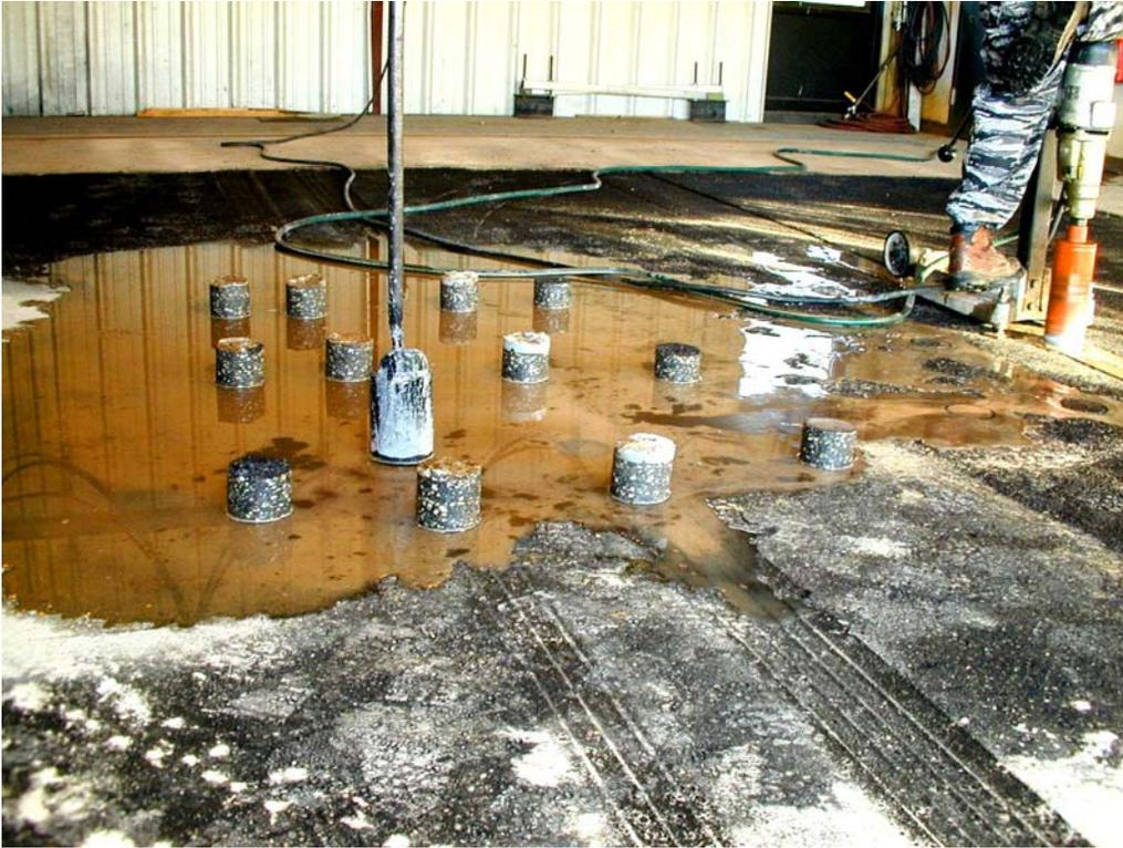
Figure D.9 Cores taken after traffic
