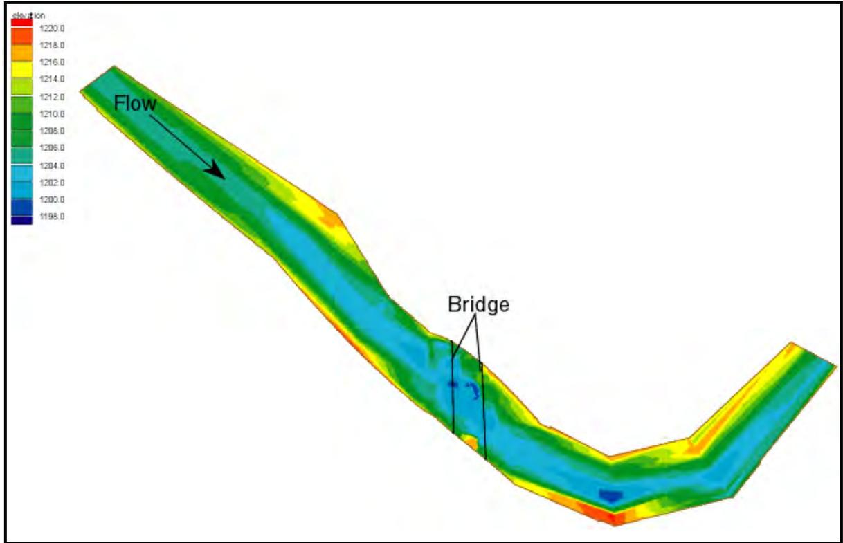
Figure 3. Bathymetric contour plot of James River in the vicinity of S.R. 37 bridge, collected during April, 2001 flood.
