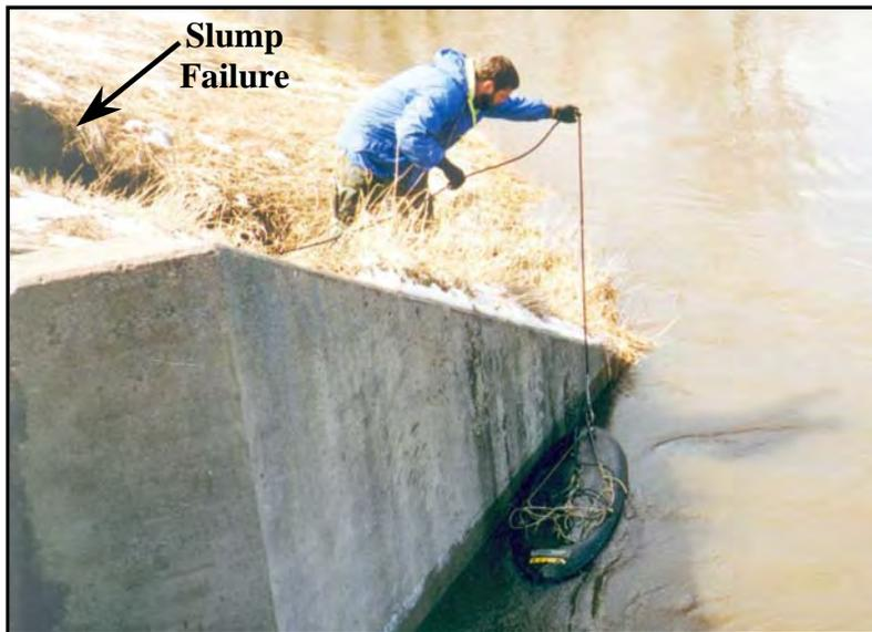
*Figure 6. Scour measurement at upstream right wingwall of U.S. 12 bridge over the Pomme De Terre River; notice slump failure of embankment.*
