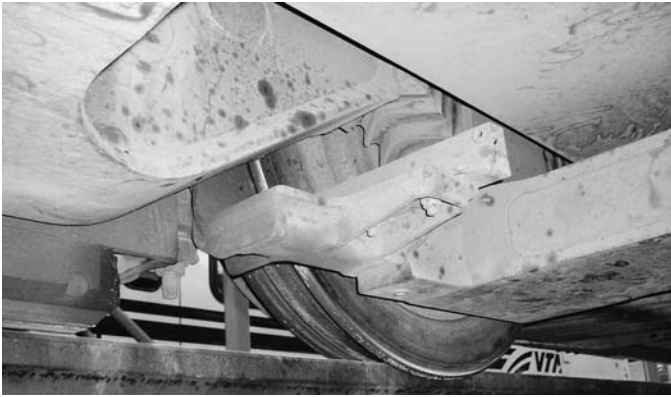
Figure 2-19. Cranked axle under the articulation (VTA Kinki Sharyo LFLRV).
