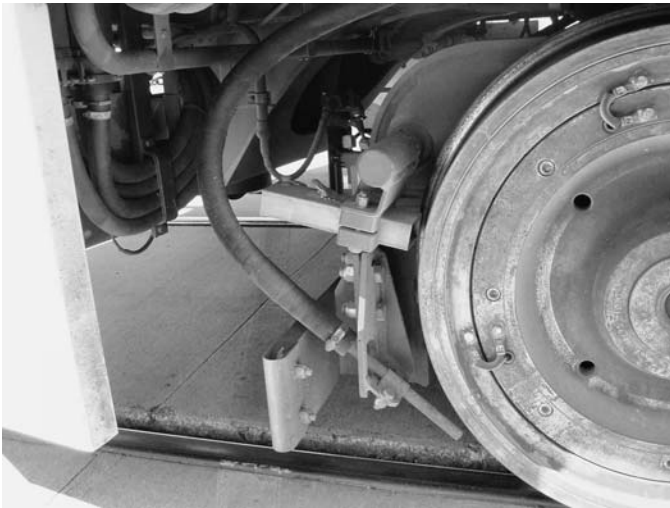
Figure 2-24. Holder for the wheel tread friction conditioner.
