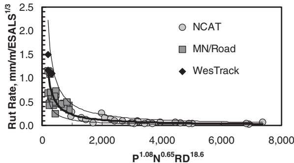
**Figure 4. Relationship Between Field Rutting Rate and Proposed Function of Resistivity,  $N_{design}$  and Air Voids; the Heavy Center Line Represents the Rutting Rate Predicted Using Equation 2 While the Thinner Lines Represent 90% Prediction Limits for New Observations.**
