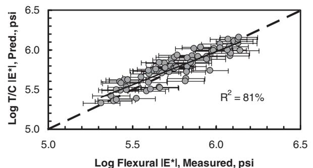
**Figure 9. Predicted Complex Modulus in Tension/Compression Compared with Measured Flexural Complex Modulus for SHRP Mixtures (Bars =  $d2s$  Confidence Limits, Solid Line = Regression Function, and Dashed Line = Equality).**
