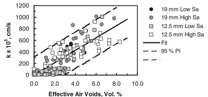
**Figure 16. Permeability of Specimens Tested During the Florida Study and During NCHRP Projects 9-25 and 9-31 as a Function of Effective Air Void Content (Solid Line = Regression Line for Predicted Permeability; Dashed Lines = 95% Prediction Interval).**
