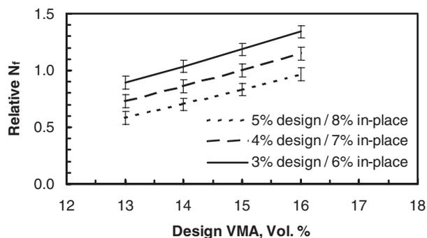
**Figure 13. Effect of Design Air Voids and Design VMA on Relative In-Situ Fatigue Life, In-Place Air Voids of 6%, 7%, and 8% for Design Air Voids of 3%, 4%, and 5%, Respectively (Errors Bars = 2s Confidence Limits).**
