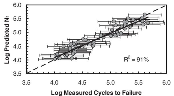
**Figure 11. Predicted and Measured Log Cycles to Failure for SHRP Flexural Fatigue Data, with d2s Confidence Limits.**
