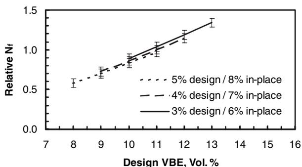
**Figure 14. Effect of Design Air Voids and Design VBE on Relative In-Situ Fatigue Life, In-Place Air Voids of 6%, 7%, and 8% for Design Air Voids of 3%, 4%, and 5%, Respectively (Errors Bars = 2s Confidence Limits).**
