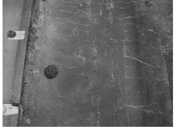
Figure 15. FA-1 test section after 2,000 wheel passes.
