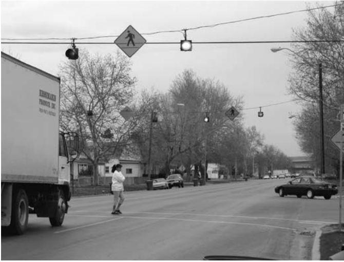
Figure 8. Pedestrian-activated overhead flashing beacon.
