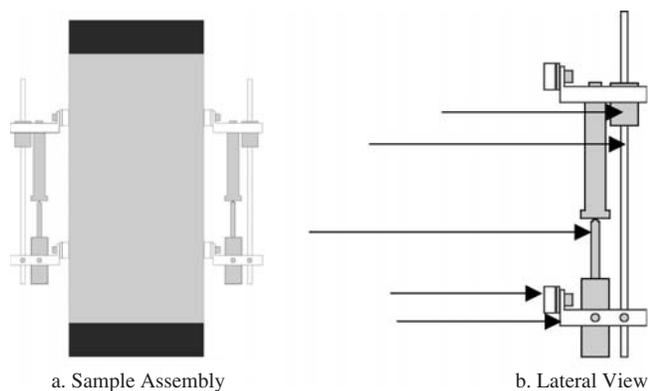
Figure 8. Specimen instrumentation of  $E^*$  testing.
