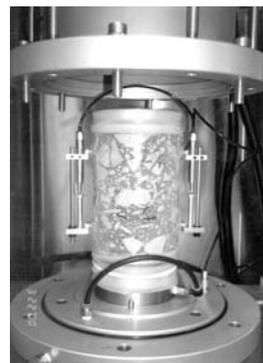
Figure 10. Confined test set-up.
