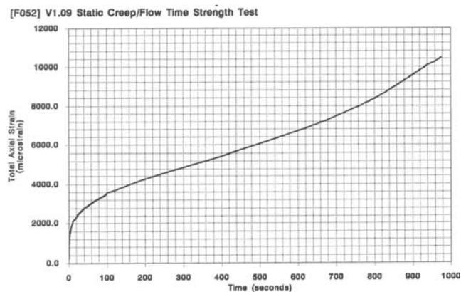
Figure 6. Total axial strain vs. time from an actual static creep / flow time test.
