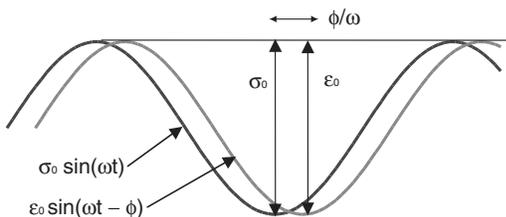
Figure 1. Dynamic (complex) modulus test.
