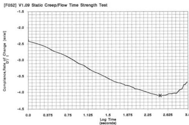
Figure 7. Typical plot of the rate of change in compliance vs. loading time.
