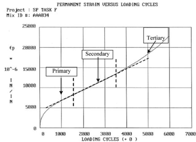
Figure 2. Typical relationship between total cumulative permanent strain and number of load cycles.
