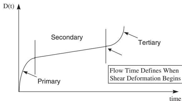
Figure 5. Typical test results between the calculated total compliance and time.
