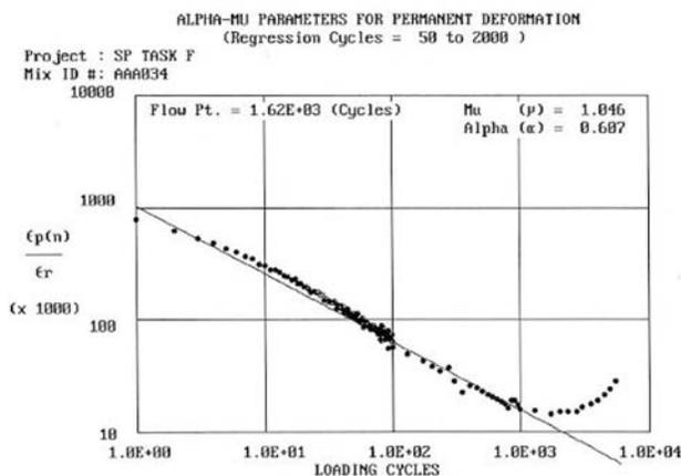
Figure 4. Permanent deformation parameters  $\alpha$  and  $\mu$  and the flow number.
