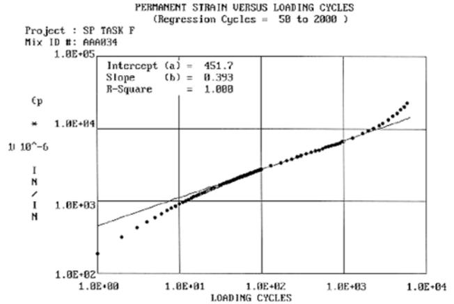
Figure 3. Regression constants “a” and “b” when plotted on a log-log scale.
