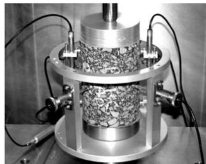
Figure 9. Vertical and radial LVDTs set-up for an unconfined test.
