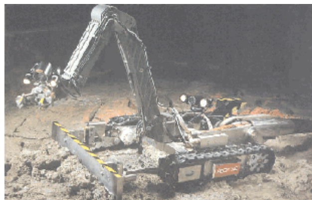
FIGURE G-4 Houdini™ in-tank crawler. SOURCE: RedZone Robotics.
