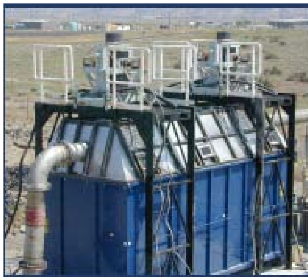
FIGURE IV-7 Bulk vitrification processing is performed in a refractory-lined commercially available container. SOURCE: AMEC Earth & Environmental, Inc.
