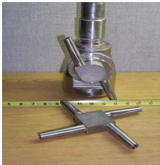
FIGURE G-1 Tank cleaning washball used at the Idaho site. SOURCE: Lockie et al., 2005.
