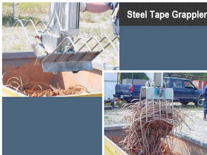
FIGURE G-11 Steel tape grappling device developed at the Savannah River Site. SOURCE: DOE-SRS, 2005g.
