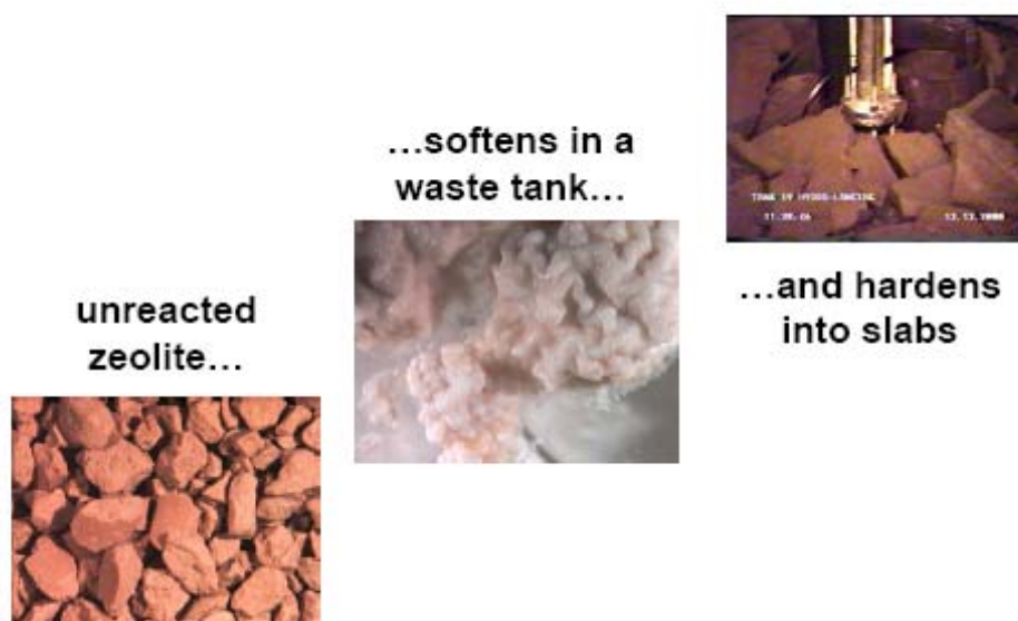
FIGURE G-8 Zeolite deposits can be difficult to remove because the fine particles formed when the slabs of zeolite are broken up by waste retrieval tools settle very quickly at the bottom of the tank. SOURCE: Caldwell, 2005a.
