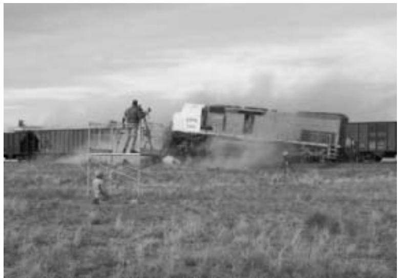
Full-scale impact test: rear-end inline collision of a locomotive with an empty flat car coupled to a stationary consist.
