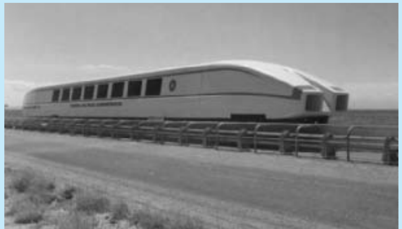
Air cushion vehicle under testing at the High-Speed Ground Test Center in the early 1970s.
