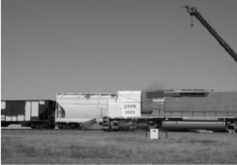
Crash test of a locomotive and trailing consist into a stationary consist.
