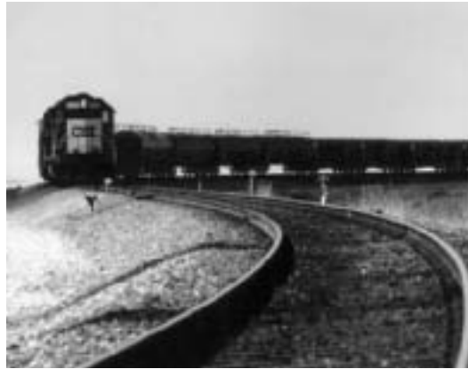
Heavy axle load test on the high-tonnage loop at the Facility for Accelerated Service Testing.
