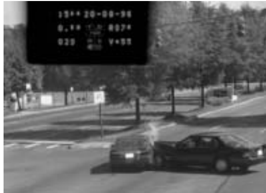
Red light running crash recorded by camera connected to traffic signal and sensors. Data include time elapsed since red signal as well as vehicle’s speed.
