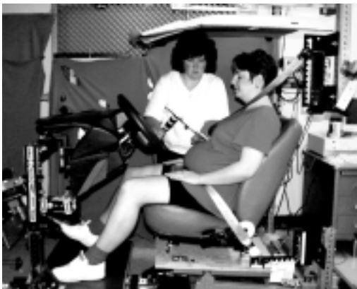
FIGURE 1 Adjustable laboratory seating buck used in study of pregnant anthropometry.
