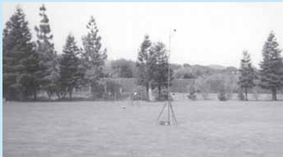
Microphones and sensors measuring traffic noise.
