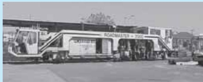
BART railgrinder used to reduce noise levels.
