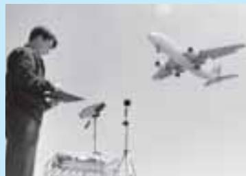
Aircraft noise has two main sources: the propeller-driven or jet engines and the airframe. Engine noise is wasted or lost energy. Only a minute portion of the engine's power radiates as noise but is sufficient to create problems for the neighborhoods around airports.
