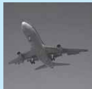
*Lowered landing gear contributes to airframe noise in flight.*
