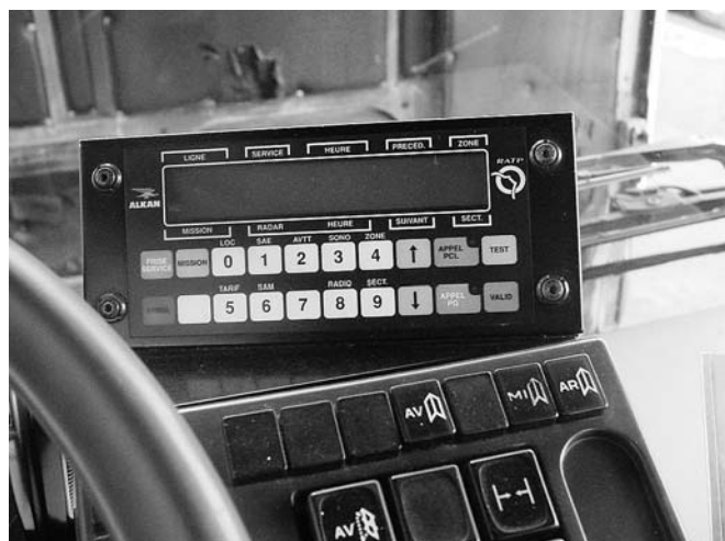
Figure 2 The On Board System that helps to monitor the maintenance needs of transit buses in Paris.
