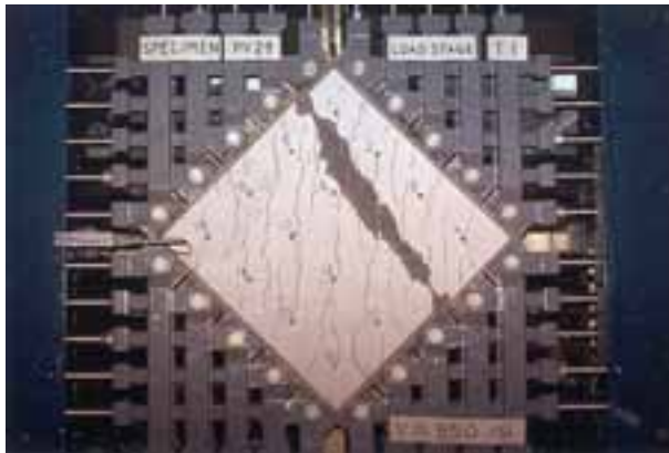
Figure A-15 Shear Panel Test (Vecchio and Collins, 1982)
