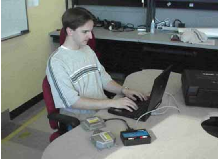
Figure 4-1. Rowan University Research Assistant downloads an EDR removed from a Saturn passenger car using the Vetronix Crash Data Retrieval System
