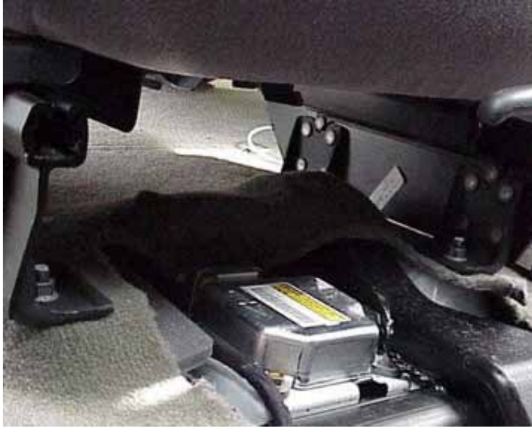
Figure 4-4. EDRs are frequently located in difficult to access locations [Kerr 2002, used with permission of the Vetronix Corporation]
