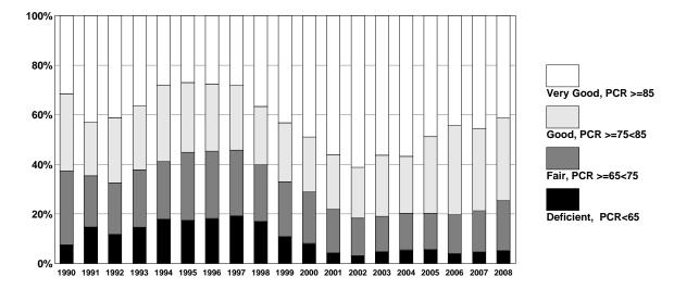
FIGURE 6 Priority system pavement conditions (statewide lane miles).
