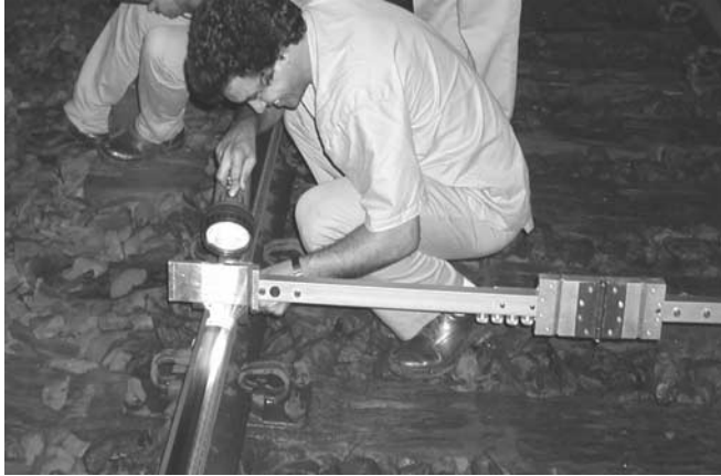
Figure 3.25. Example of ground rail template, “bar gage” and measurement.
