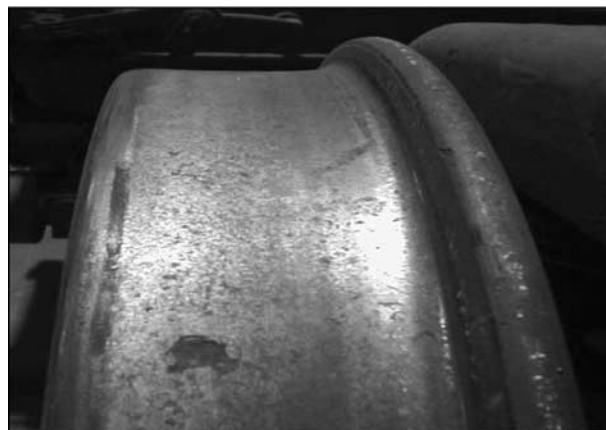
Figure A-15. SEPTA cylindrical wheel wears into slightly hollow, but stable shape on Suburban Route 101, LRV.
