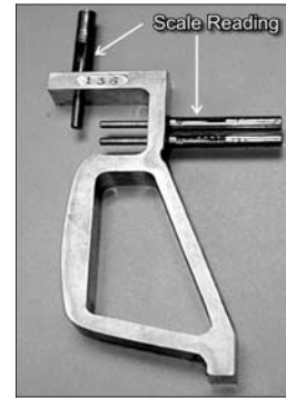
Figure 3.5. Measuring gage for AREMA 136 RE rails.
