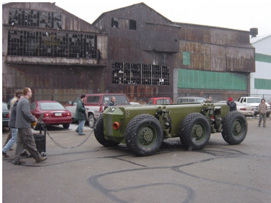
FIGURE 6.4 The Spinner, from Carnegie Mellon University, with turbine power, electric final drives, and long-travel suspension. SOURCE: Available online at < http://www.darpa.mil/body/team_spinner.htm >. Last accessed on March 31, 2004.
