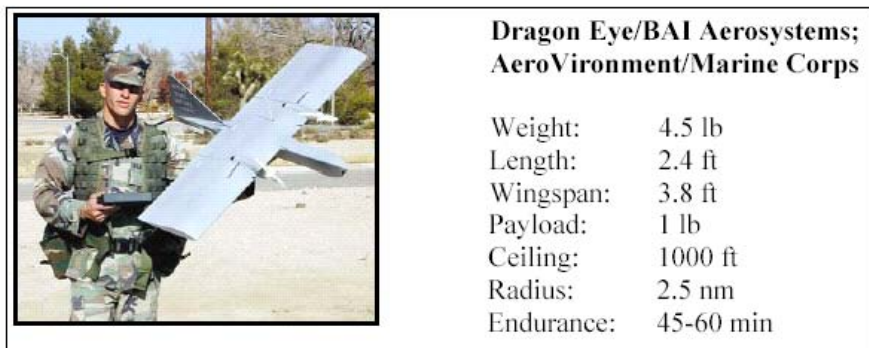
FIGURE C.5 Dragon Eye. SOURCE: Office of the Secretary of Defense. 2002. Unmanned Aerial Vehicles Roadmap 2002-2027 , Department of Defense, Washington, D.C., December, p. 10.
