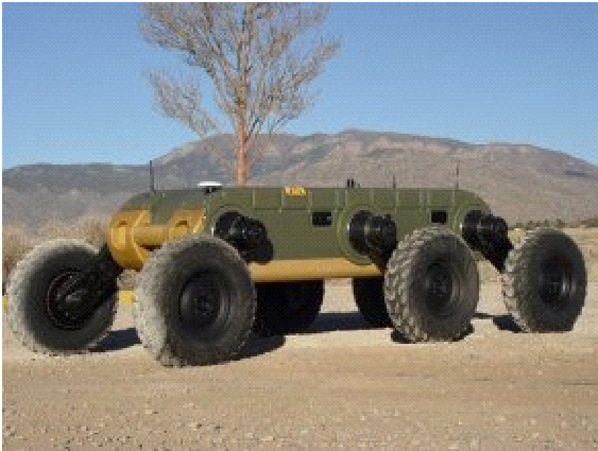
FIGURE 6.3 The Retarius vehicle from Lockheed Martin, featuring active articulated suspension. SOURCE: Defense Advanced Research Projects Agency.
