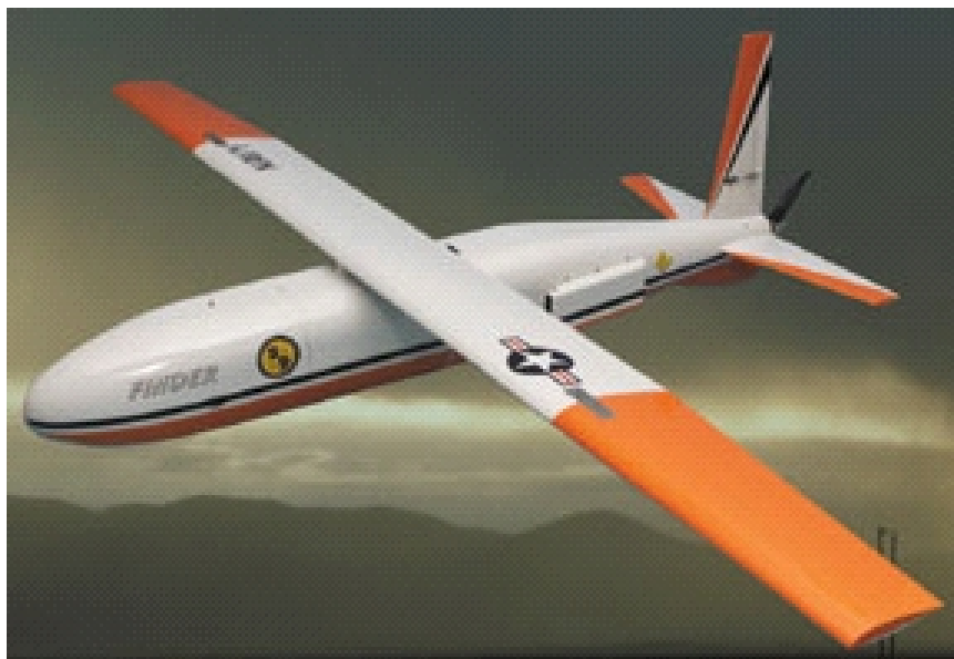
FIGURE B.2 The Finder unmanned aerial vehicle developed by the Naval Research Laboratory has a folding and pivoting wing to stow in a “cigar-tube” shape. SOURCE: Office of the Secretary of Defense. 2002. Unmanned Aerial Vehicles Roadmap 2002-2027 , Department of Defense, Washington, D.C., December.
