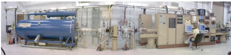
FIGURE 2.5 Nuclear microprobe at the Center for Accelerator Mass Spectrometry at the Lawrence Livermore National Laboratory. Courtesy of the Center for Accelerator Mass Spectrometry.
