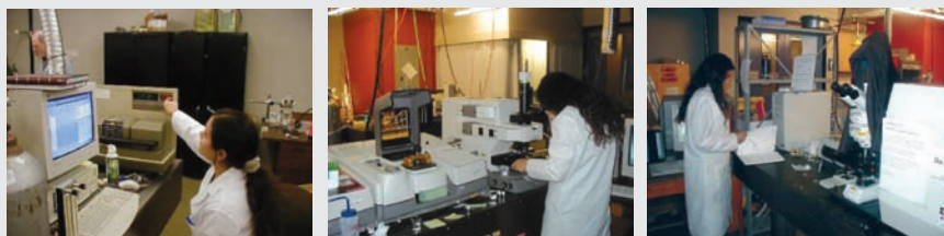
FIGURE 2.2.1 Several instruments included in the Rice SEA are (left to right) a thermogravimetric analyzer with infrared spectroscopy, a Fourier transform infrared microscope, and a Raman microscope. Courtesy of Rice University Shared Equipment Authority.
