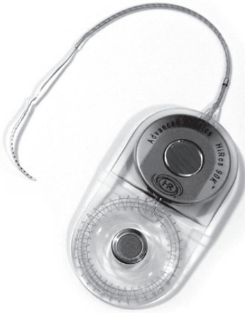
FIGURE F.3 An implanted receiver and electronics package. (Courtesy of Advanced Bionics Corporation.)
