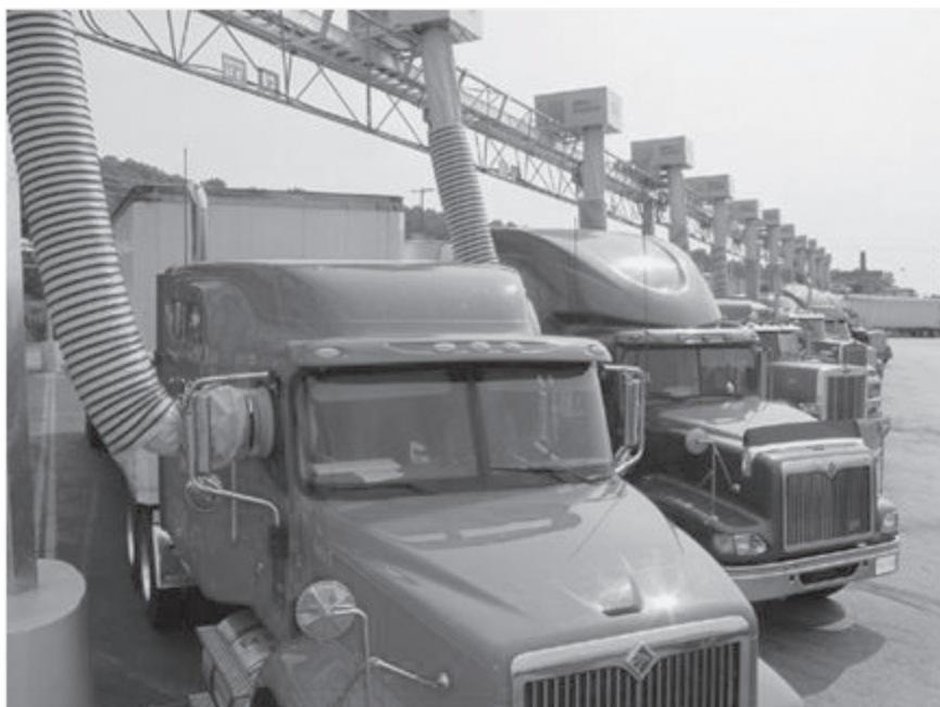
FIGURE 3.3 Reducing engine idling by providing electrical access at truck stops is one measure to decrease emissions. SOURCE: Idle Aire. Reprinted with permission.
