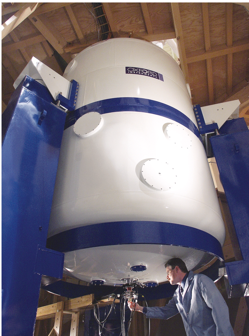
FIGURE 2.6 The magnet of the 900-MHz NMR spectrometer in Pacific Northwest National Laboratory's Environmental Molecular Sciences Laboratory. This picture illustrates some of the issues associated with high-field magnets. This 21-T magnet was manufactured by Oxford and has a 63-mm room-temperature bore and a stored energy of 27 MJ; it is sited inside a cylindrically shielded enclosure 24 ft in diameter and extends 15 ft above and below the main laboratory floor (the magnet itself is 8 ft in diameter and 21 ft tall). The center of the magnetic field is located at exactly floor level to preserve the desired symmetry of the magnet and shield. The person standing next to the magnet is just over 6 ft tall. Photo courtesy of William R. Wiley Environmental Molecular Sciences Laboratory, Pacific Northwest National Laboratory.
