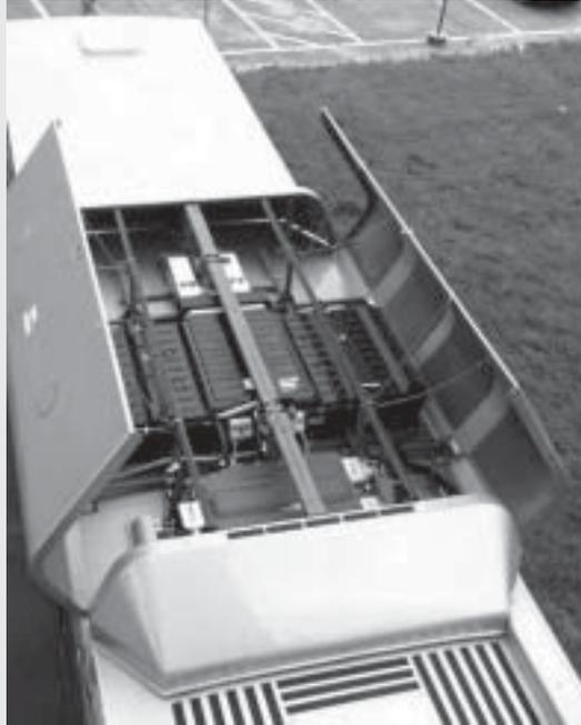
Electric storage system of a hybrid gas–electric bus, now being tested by CTTransit in Hartford, Connecticut.
