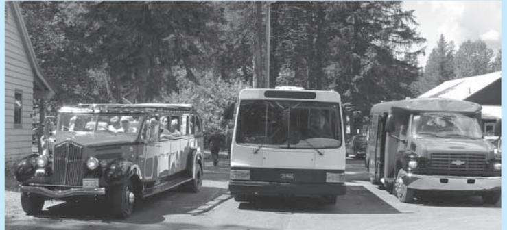
*National Park Service and Federal Highway Administration are investigating potential vehicles for shuttle service in Glacier National Park, as a complement to the interpretative tours given by the refurbished red buses (left). Two prototypes include a hybrid electric vehicle (center) and a wheelchair-compliant, propane-fueled bus (right).*
