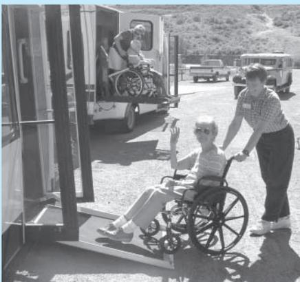
The entry ramp in the low-floor, new yellow bus extends to accommodate passengers in wheelchairs.
