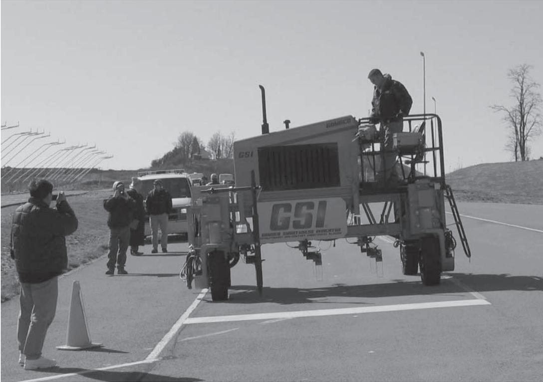
The GSI profiler uses sonic technology to measure pavement.
