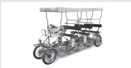
Four-wheeled, pedal-powered cycle
