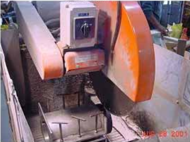
FIGURES 1 through 4 Initial steps in cutting gyratory pill to obtain test specimens.
