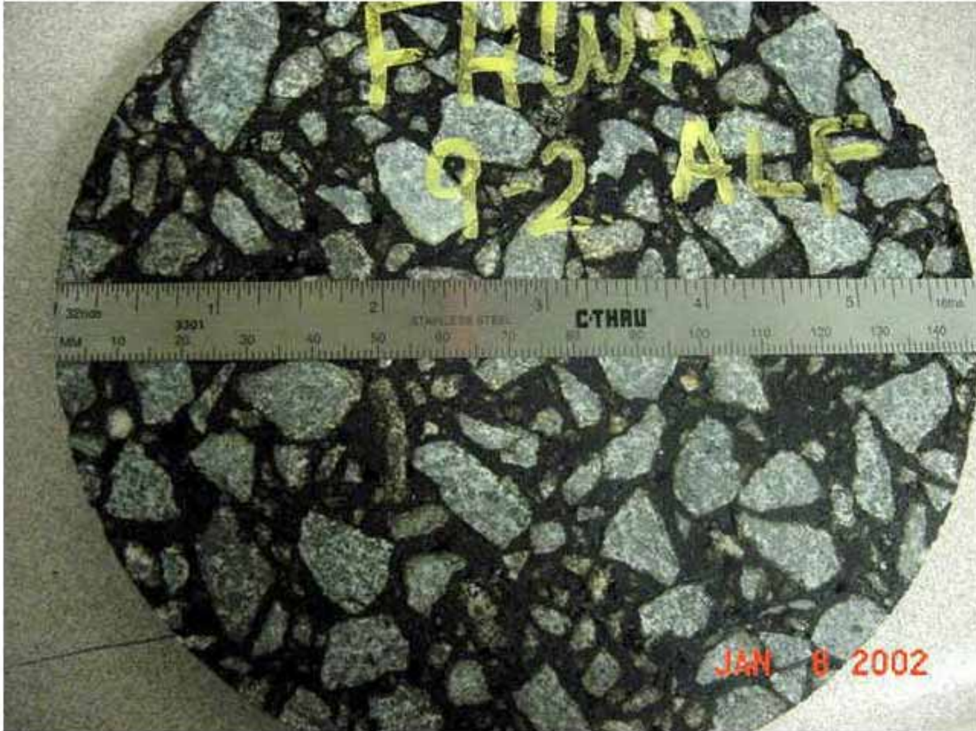
FIGURE 20 Aggregate structure of FHWA ALF mixture.
