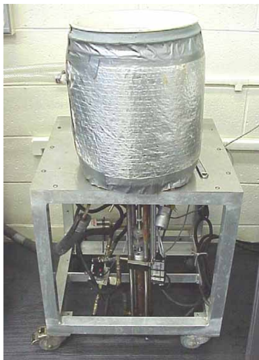
FIGURE 2 Portable test assembly: servohydraulic actuator (below) and temperature bath (above).
