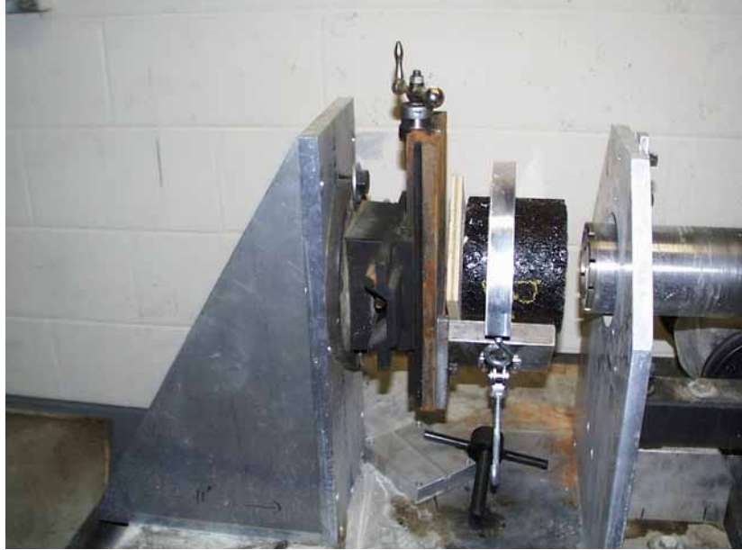
FIGURE 3 Coring fixture at Advanced Transportation Research and Engineering Laboratory to produce 100-mm cavity in standard gyratory specimen.
