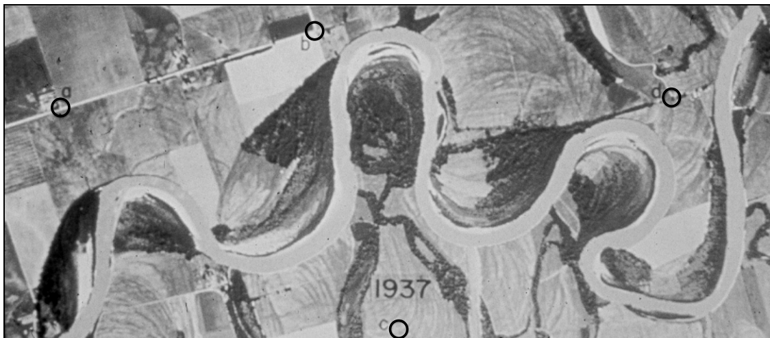
Figure 34. Aerial photograph of a site on the White River in Indiana showing four registration points (circles designated a through d) common to the 1966 aerial photo.
