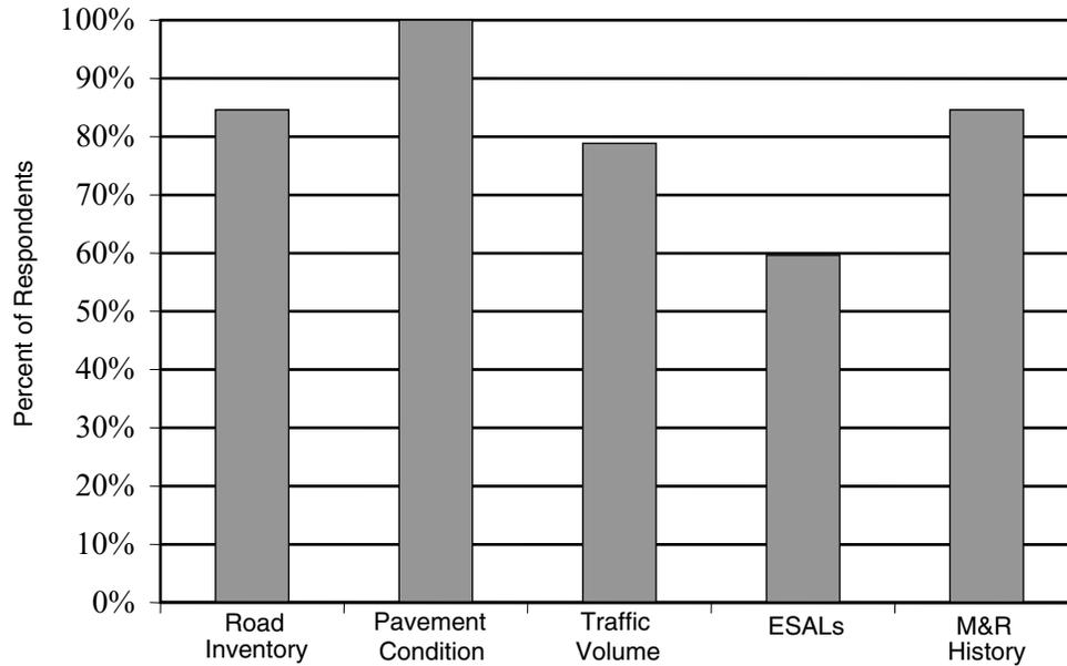
FIGURE 1 Types of pavement management data collected.
