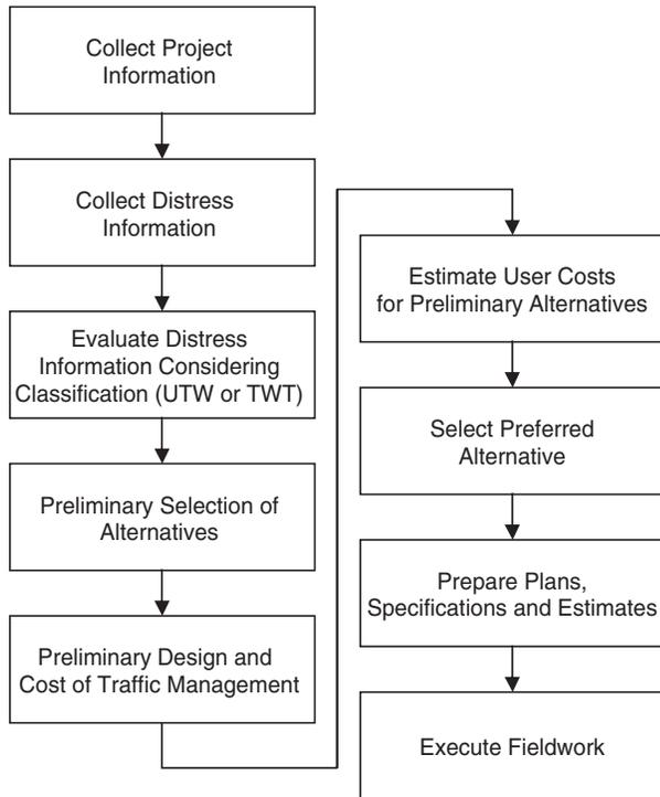
FIGURE 29 Flowchart for evaluating recommended rehabilitation activity (57).
