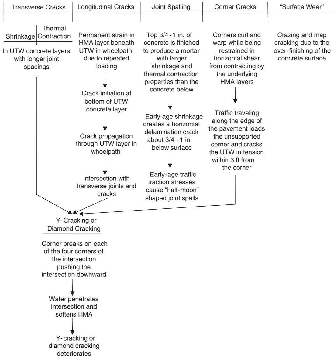
FIGURE 28 Fault tree indicating distress development for UTW (2).
