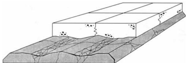
FIGURE 17 With an uneven HMA, err on the thick side (82).
