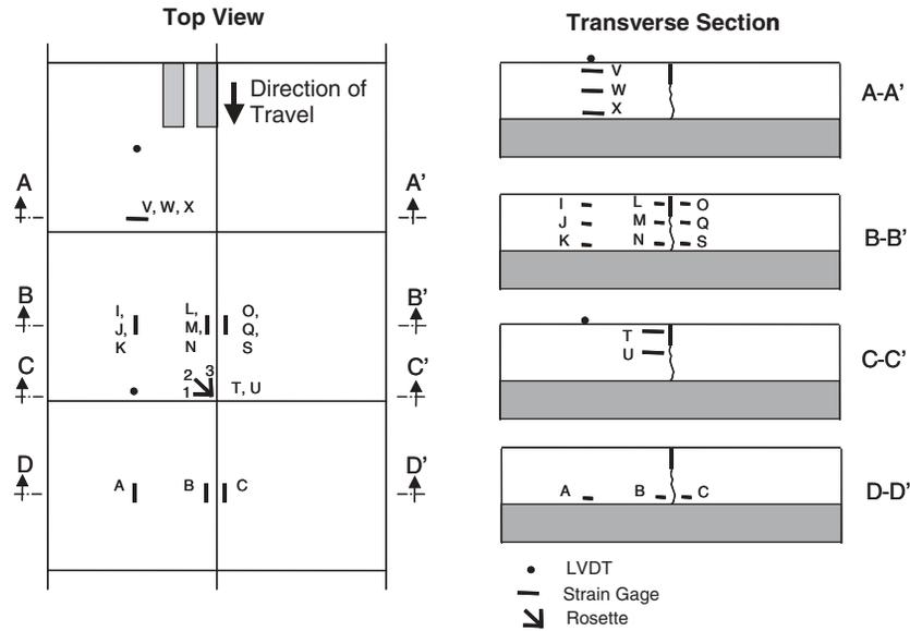
Note: Gauges A, B, and C were installed only in Lane 5. LVDT = linear variable displacement transducer.
