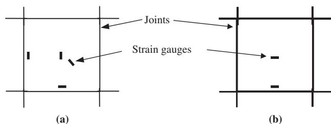
FIGURE B6 Plan view of the location of embedment strain gauges: (a) typical pattern; (b) pattern for slabs with four free edges.
