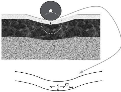
FIGURE B20 Mid-slab cracking mechanism in a UTW slab.
