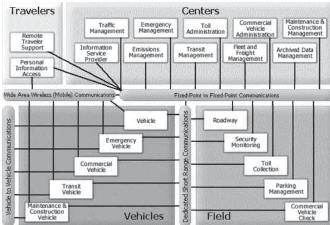
Schematic view of National ITS Architecture, Version 5.0. (Source: [itsarch.iteris.com/itsarch/html/entity/paents\\_b.htm](http://itsarch.iteris.com/itsarch/html/entity/paents_b.htm).)
