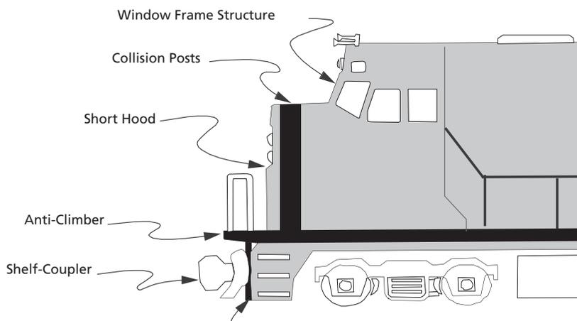
FIGURE 4 Locomotive components considered for design modification.
