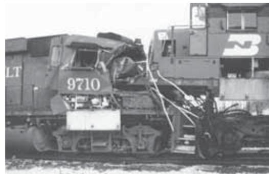
Scenario 1 locomotive crash near Smithfield, West Virginia, August 20, 1996—collision with a 28-car train traveling at 24 mph caused the trailing locomotive of a 41-car train traveling at 22 mph to override the leading locomotive.
